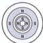
Outer magnets are rotated by a direct coupled motor, thus rotating inner magnets and rotor shaft.
